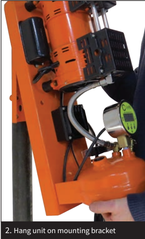
2. Hang unit on mounting bracket
