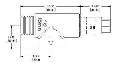
\* Note: Valve showing in the fully open position. Model LVAPR is factory set a approximately 185 psi
